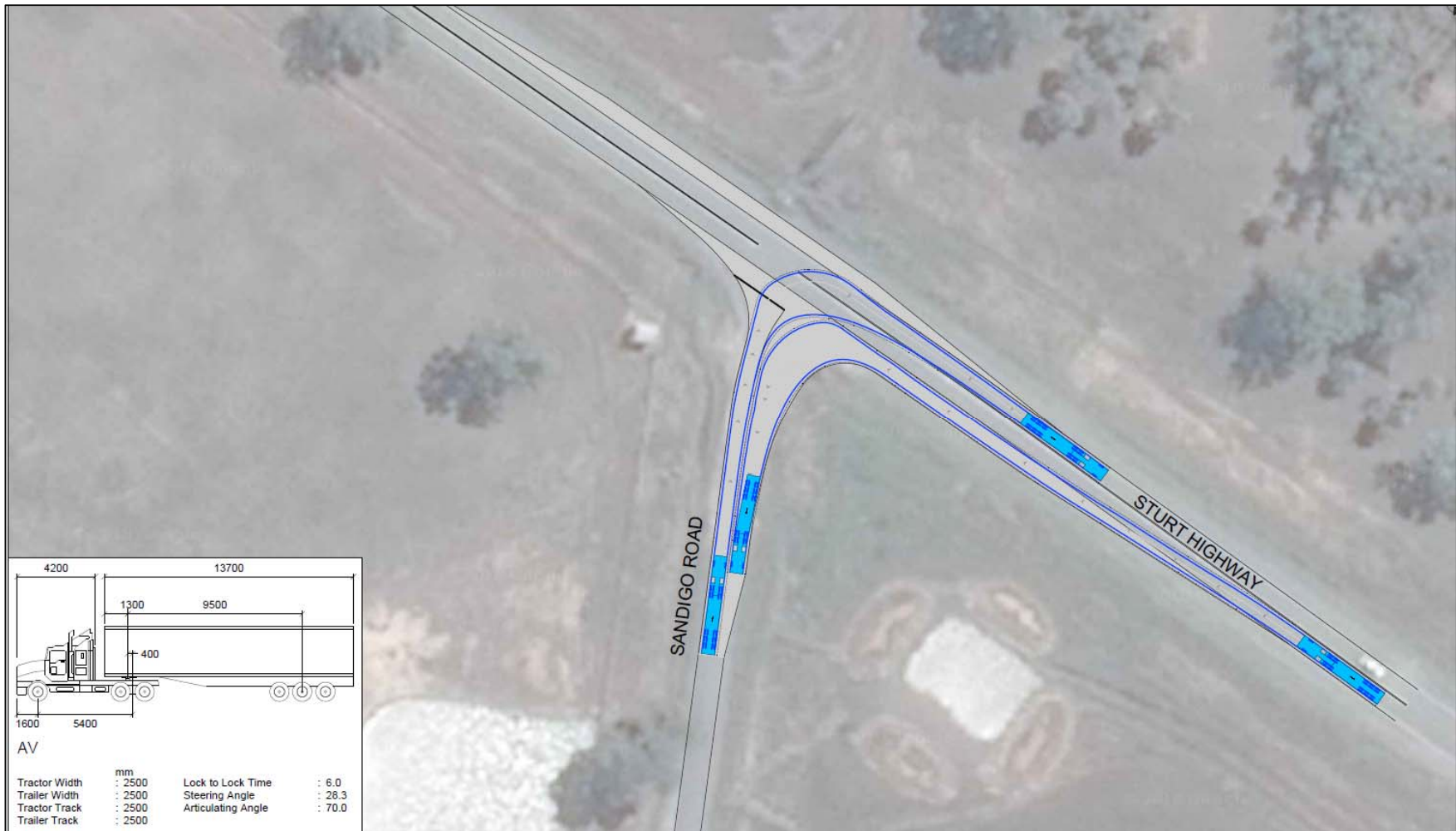
Figure 3-17 Proposed AV right hand turn from Sandigo Road to Sturt Highway
