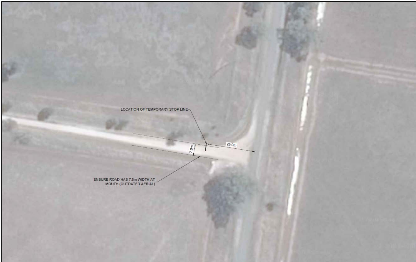
Figure 3-18 Proposed intersection treatment at Muntz and Sandigo Road
