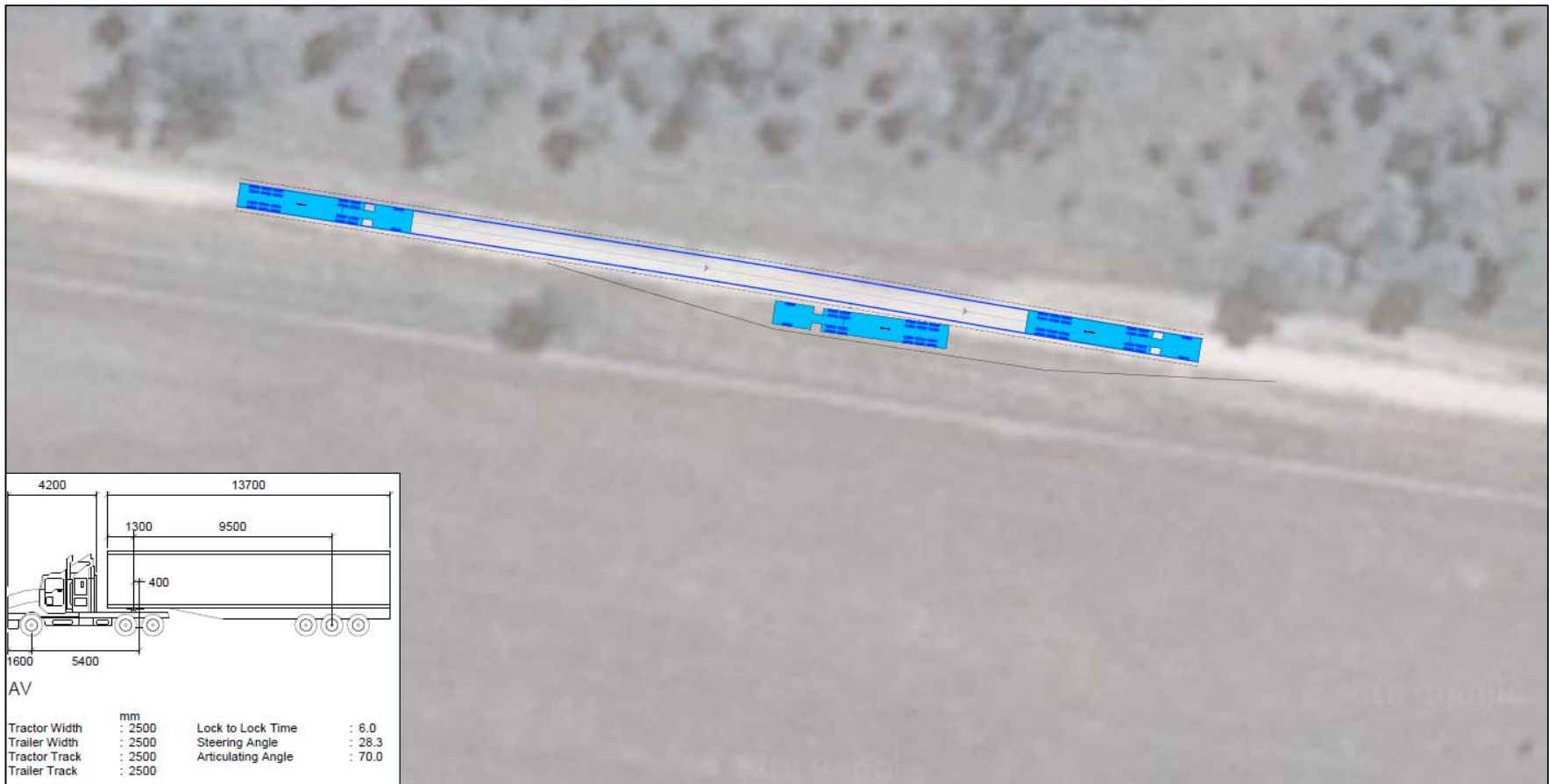
Figure 3-14 Proposed passing lanes and AV movements on Muntz and Sandigo Roads
